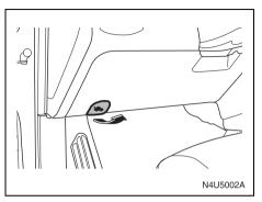
1) Pull the hood release handle located at the lower left side of the instrument panel.
